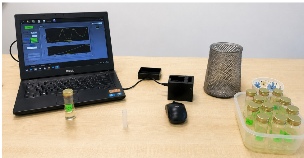
Figure 1. Experimental setup for MicroNIR spectral data acquisition.
