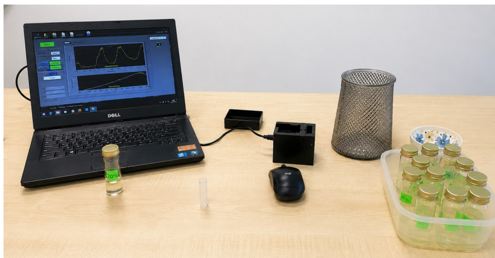
Figure 1. Experimental setup for MicroNIR spectral data acquisition.
